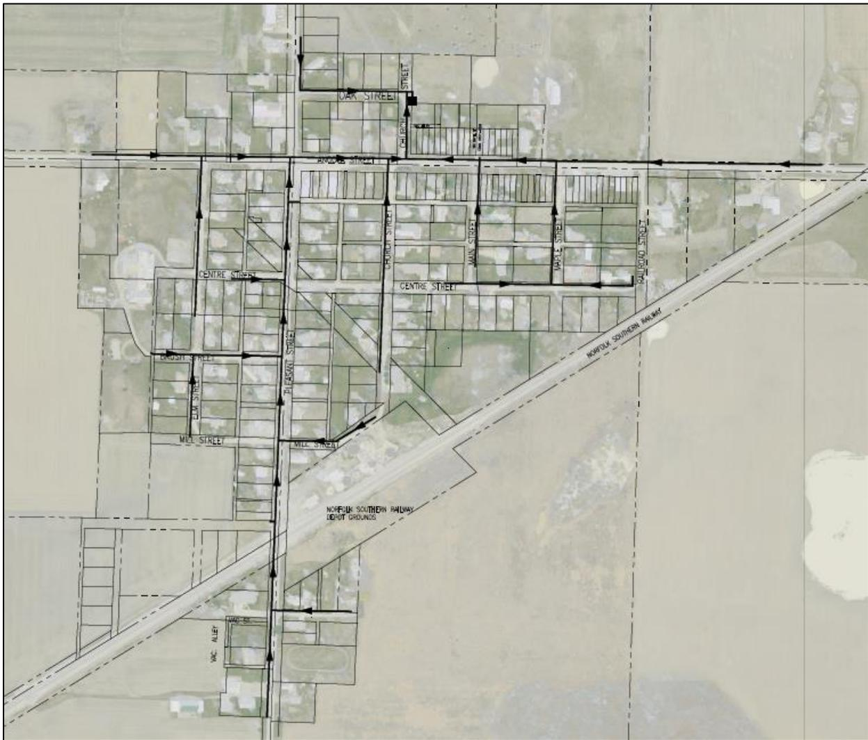
**Figure 4. Map of new gravity sewer alignment along streets in Kunkle and new pump station marked with black square on Church Street.**
